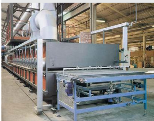
Tile conveyor in ceramic plant
