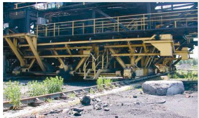
Transfer car undercarriage with drive arrangement
