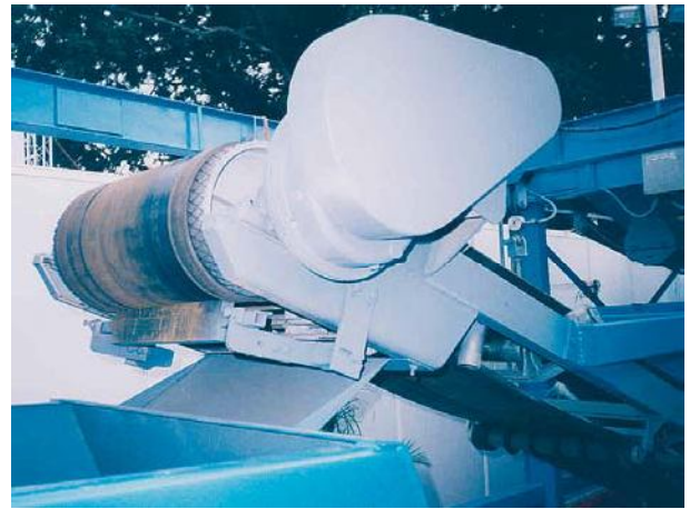
Feed conveyor in batching plant
